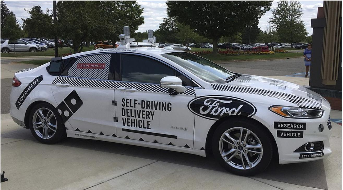
This photo shows the specially designed delivery car that Ford Motor Co. and Domino's Pizza will use to test self-driving pizza deliveries. The car can drive itself, but it will have a backup driver. It lets customers tap in a code and retrieve their pizza from a warming space in the back seat. Photo from: AP Photo/Dee-Ann Durbin.
